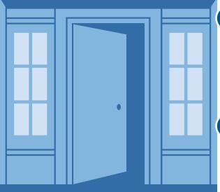
**CLEANING SURFACES: Clean** the door and door jamb to be weather stripped. For best results, weather stripping should be applied to clean, dry surfaces above 20° Fahrenheit.
