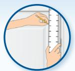
Save energy and seal air leaks by weather stripping exterior doors. How do you know if you need to weather strip? If you can see any amount of light between the door frame and the floor, weather stripping should be applied to eliminate energy waste. This DIY energy-saving project is relatively easy and inexpensive depending on the type of materials selected. The most common weather stripping material is self adhesive foam strips, although rubber, vinyl, metal, or a combination of materials
