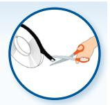
**APPLYING:** Apply one continuous strip snugly along each side, making sure it meets tightly at the corners. The material should compress tightly between the door and door jamb, without making it difficult to shut.
