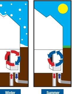
moves the solution into the dwelling's heat pump. Within the heat pump, a heat exchanger removes the heat from the water solution, concentrates the heat and then distributes the heat throughout the buildina.
