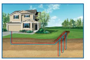
Vertical installations, where well drilling equipment is used, are generally more expensive, but are ideal where land area is limited.
